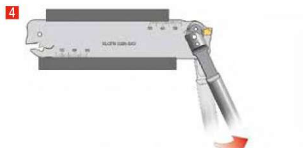
4 Moving the key forward causes the insert seat to close and clamp the insert.
