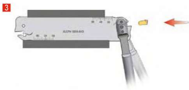
3 Load the grooving insert into position and press against the seat.
