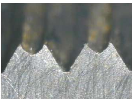
Underformed – core hole too large
